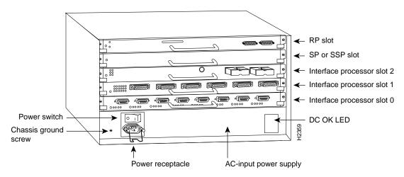
The Cisco 7505 is a five-slot model that provides four interface processor slots. Figure 2 shows the interface processor end of the Cisco 7505. The Route Switch Processor (RSP1), which is a required system component in the Cisco 7505 router, occupies the top slot. The remaining four slots support any combination of interface types: Ethernet, Token Ring, FDDI, and so forth.
